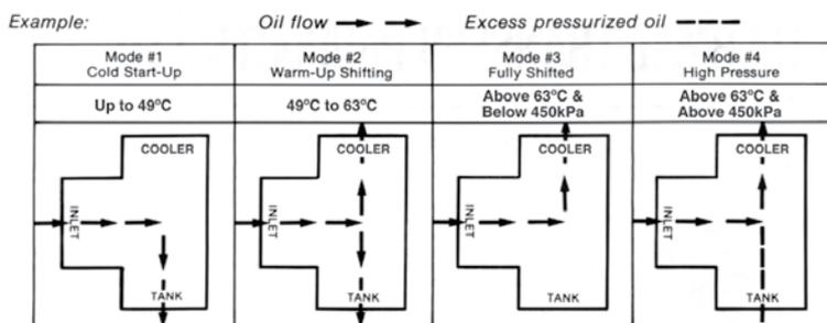
NOTE: If the temperature drops below 63°C the valve will shift back to modes 2 or 1.
